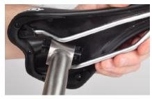
Step 5) Slide seat post head with upper cradle between the rails of the saddle. Start from the back of the saddle with post rotated 90°.
