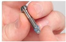
Step 4) Apply grease to the threads of the bolt and insert the bolt into the non threaded wedge. You'll need this in step 9.
