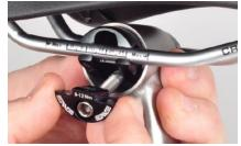
Step 9) With your other hand, pick up the right side wedge w/ bolt and line it up with the left wedge. Pinch assembly to hold it all in place.
