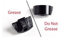
Do not grease the bottom of the wedges that interface with the seat post barrel. This can cause saddle slipping issues.
