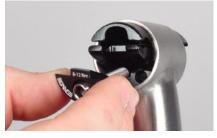
Step 1) Disassemble your seat post by loosening the bolt and removing the 2 wedges.
