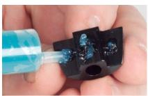
Step 3) Apply very light coating of grease to each sliding wedge interface. You'll need these in step 8. (\*\*\* See Note.)
