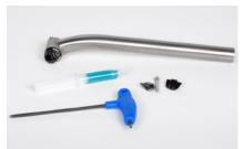
Tools needed: 5mm Allen Wrench, Torque Wrench, Synthetic Grease (very small amount)
