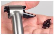
Step 2) Remove lower rail cradle. Leave upper cradle installed in post head.
