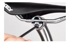
Step 10) Begin to tighten. Adjust saddle angle and position. Once desired position is achieved, tighten bolt to 8-12 Nm (71-106 in-lbs, 5.9-8.8 ft-lbs)
